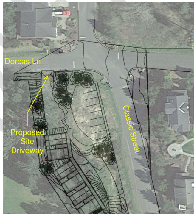
Driveway Location Relative to Intersection Markings (Site Plan Excerpt Over Satellite Photo)
