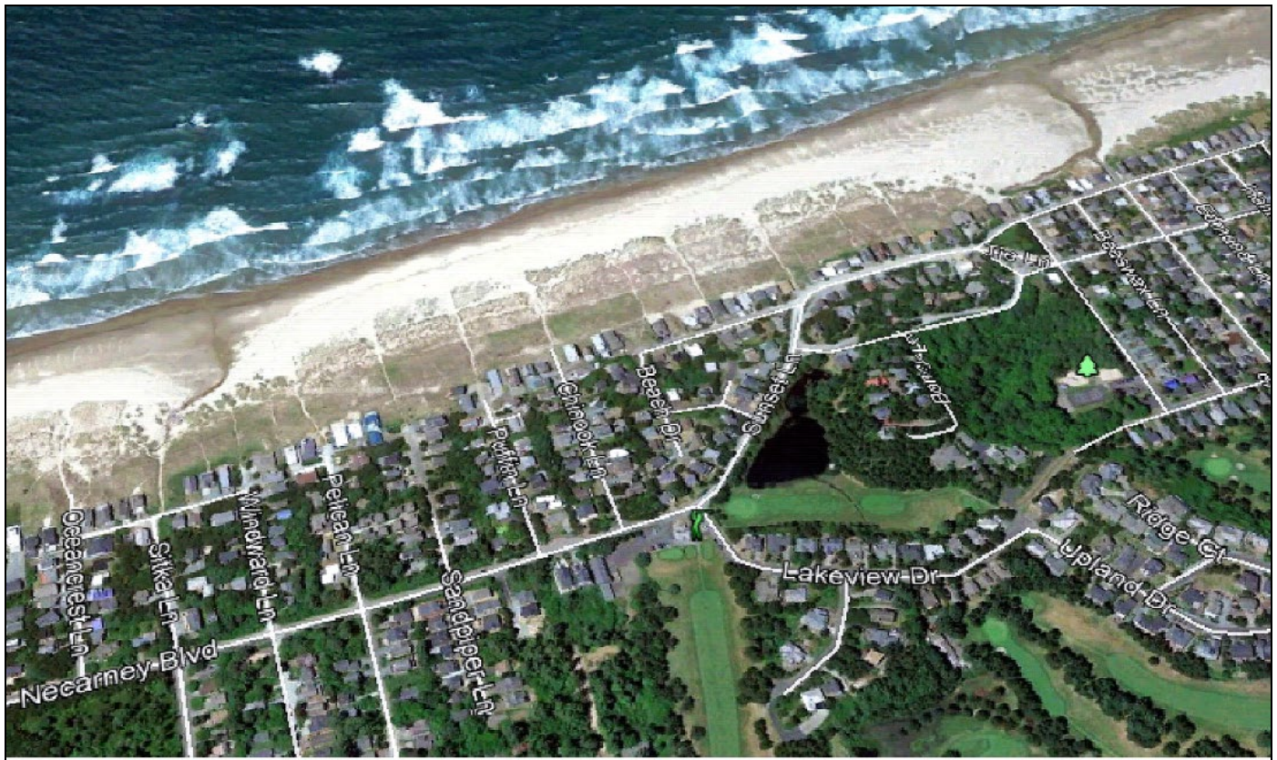
Figure 15: Creek channels crossing the beach allow surf easy access to the upper beach and facilitate rip cell embayment formation, as shown in this aerial view. Note the northward deflection of the channels, caused by heavy sand deposition during winter southwesterly storms. The rip cells are as much as 1000 ft wide. The southern rip cell created a large open area where driftwood accumulated and is now buried by sand.
