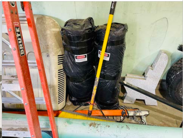
Building 3: Stored/bagged presumed asbestos-containing materials
