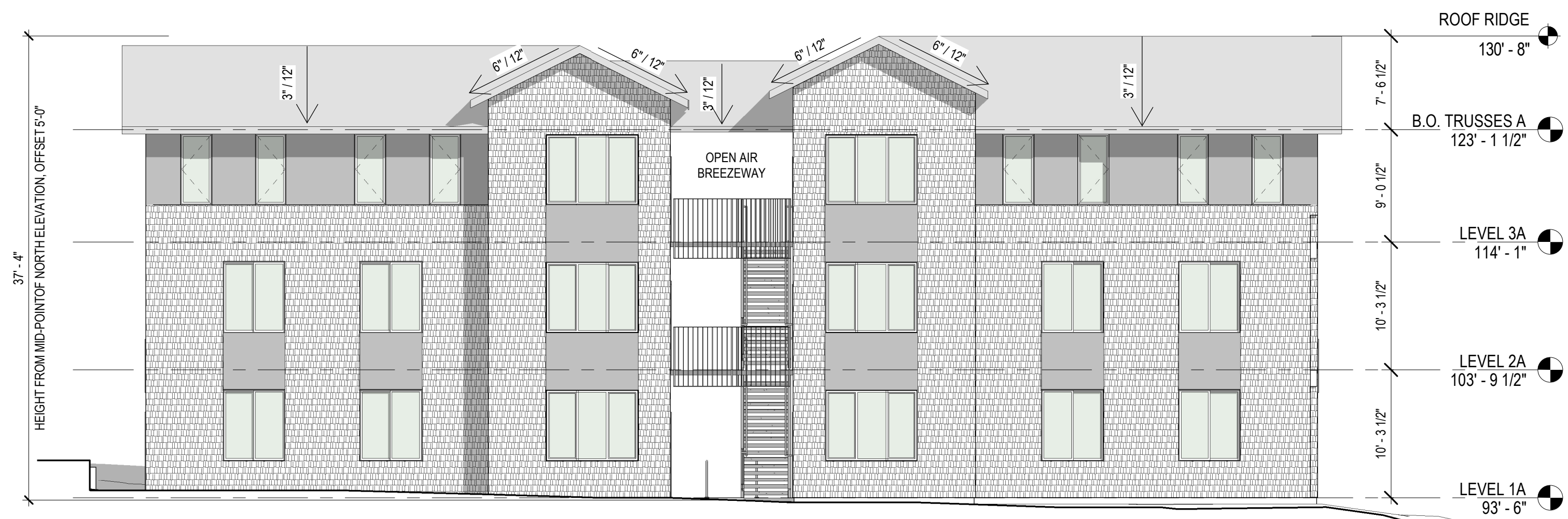
A21 2 BUILDING A - NORTH ELEVATION SCALE: 1/8" = 1'-0"
