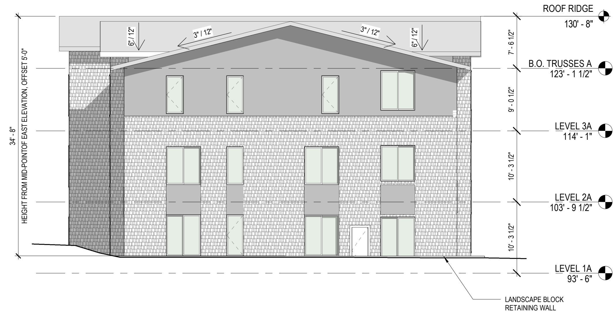
A21 1 BUILDING A - EAST ELEVATION SCALE: 1/8" = 1'-0"
