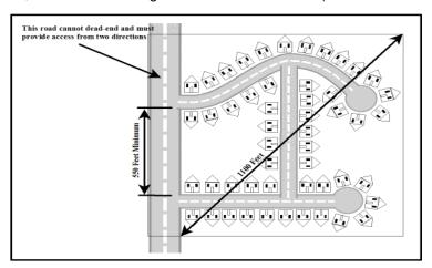
FIRE APPARATUS ACCESS ROAD WIDTH AND VERTICAL CLEARANCE: Fire apparatus access roads of 150-feet or greater shall have an unobstructed driving surface width of not less than 20 feet (26 feet adjacent to fire hydrants (OFC D103.1)) and an unobstructed vertical clearance of not less than 13 feet 6 inches. (OFC 503.2.1 & D103.1)
