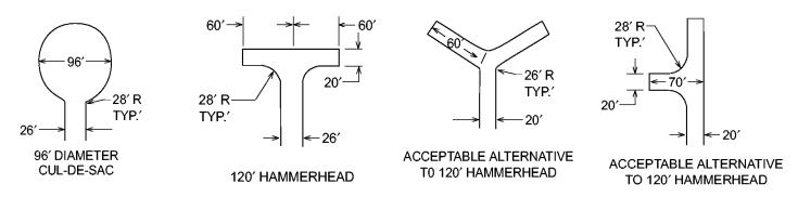
**TURNING RADIUS:** The inside turning radius and outside turning radius shall be not less than 28 feet and 48 feet respectively, measured from the same center point. (OFC 503.2.4 & Appendix D)
